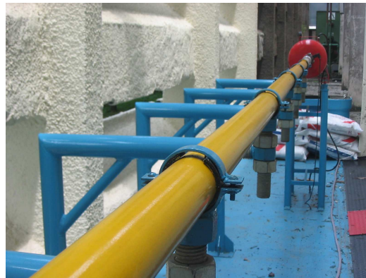
Figure 3. GMSIE's gas gun projectile launcher.
