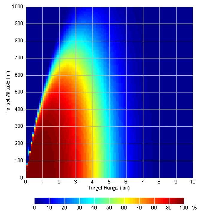
Carrier Frequency 3050 MHz **PRF** 1.9 kHz 60 KW Peak Power Pulse Length 80 ns Inst. Bandwidth 12.5 MHz 4 m Antenna Altitude Transmit Gain 26.8 dBi 1.80 ° Azimuth Beamwidth : Polarization Η Doppler Processing none Number of Bursts 9 False Alarm Prob. : 3e-006 Free space OΠ Target RCS  $0.01 \, \text{m}^2$ Swerling Case
