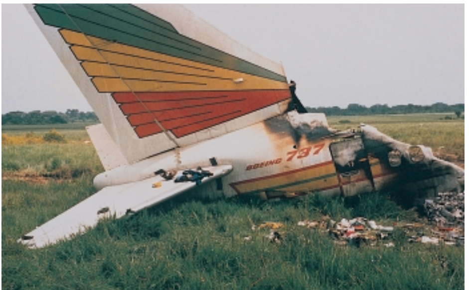
Remains of the Boeing 737 that collided with a flock of pigeons and crashed on 15 September 1988, in Ethiopia. 35 of the 104 passengers were killed.
