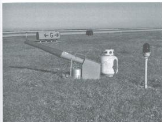
Fig. 4.2. Propane exploders have long been used to repel birds by simulating the sound of a shotgun blast, which is thought to represent a threat to birds. Photo credit: Thomas W. Seamans
