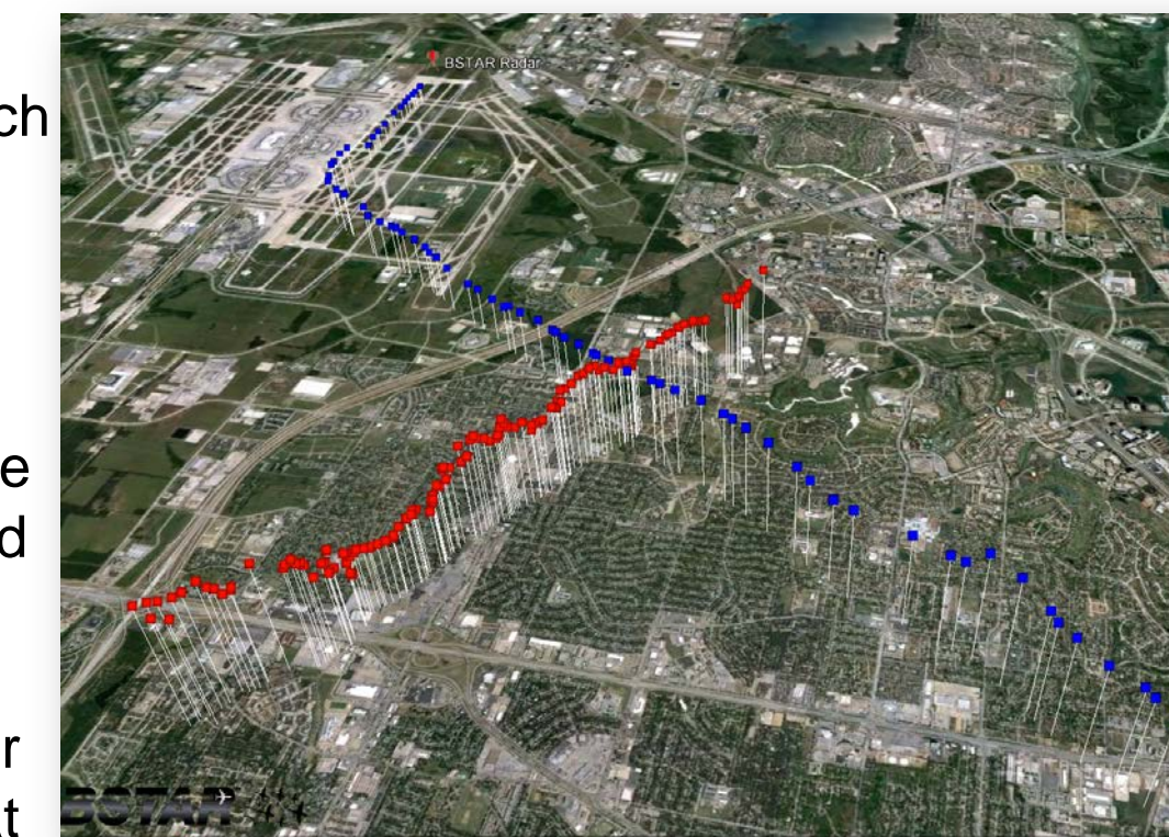
Miss distance monitor detects an actual near-miss of bird and aircraft
