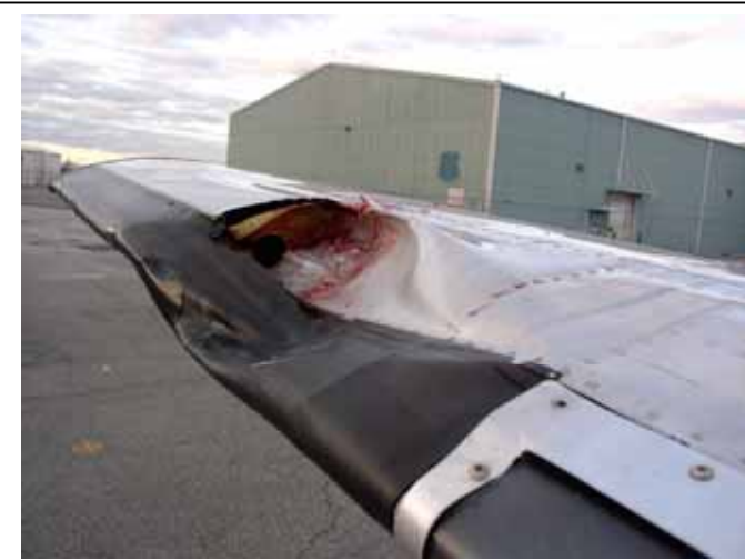
This SA227 Metroliner struck a common goldeneye (a 2.2-lb duck) at 600 feet AGL on departure from a western USA airport on 2 March 2006. The bird penetrated right wing of aircraft. Pilot declared an emergency, returned to airfield and landed without incident. Aircraft required extensive repair. Feather remains were sent to the Smithsonian Institution where the species was identified.
