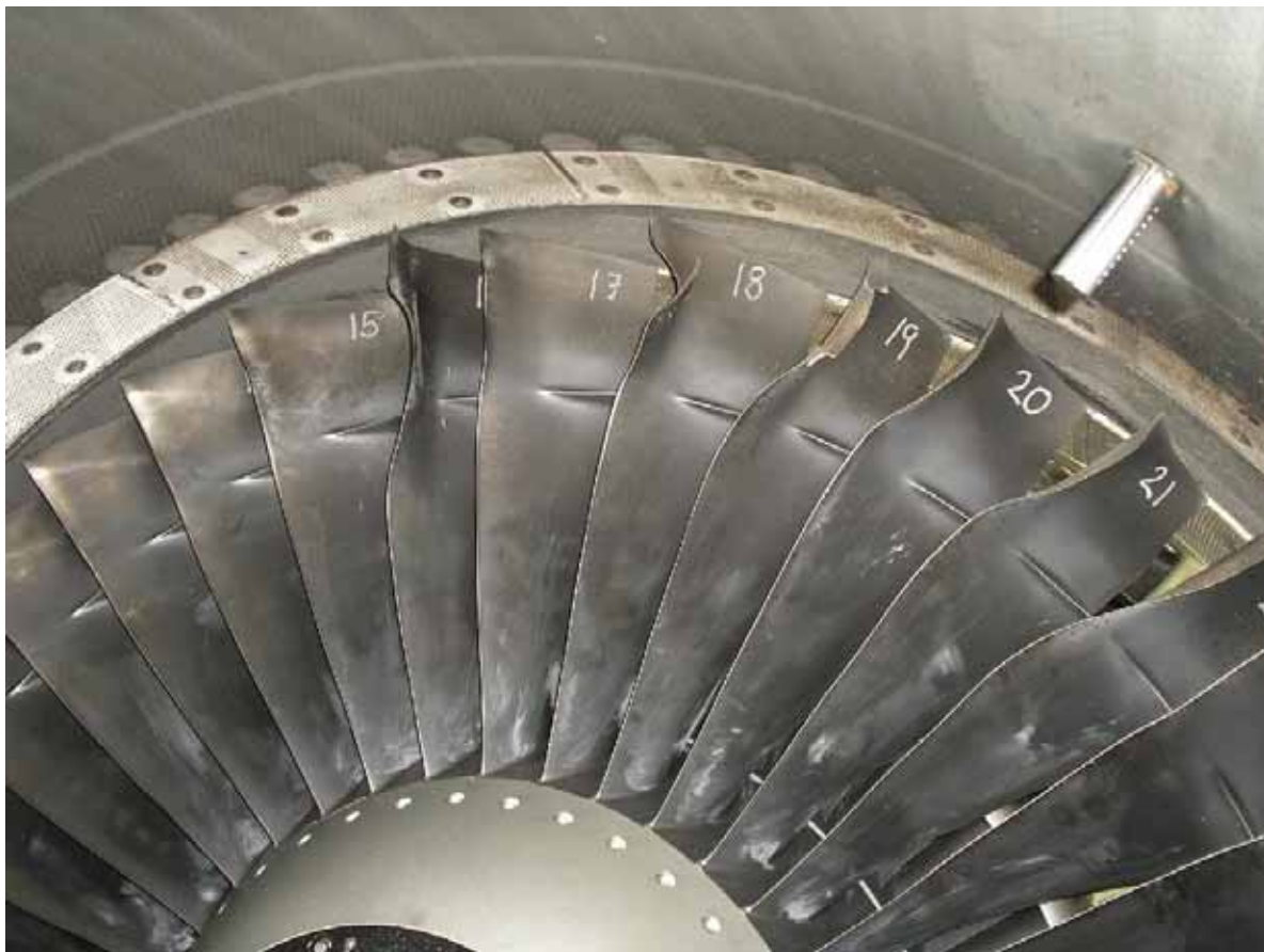
A great horned owl was ingested into the #2 engine of a Boeing-737 departing a western USA airport on 26 November 2006 at 0048 hours. The pilot had to shut the damaged engine down and make an emergency landing with 1 engine.
