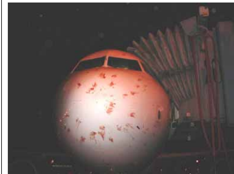
An Airbus 320 on final approach at an eastern USA airport on 1 March 2006 flew through a large flock of European starlings at 100 feet AGL, resulting in multiple strikes to the front of aircraft including both engines. Over 270 starling carcasses were removed from the runway threshold. The #1 engine was removed to repair damage. The aircraft was out of service for 24 hours.
