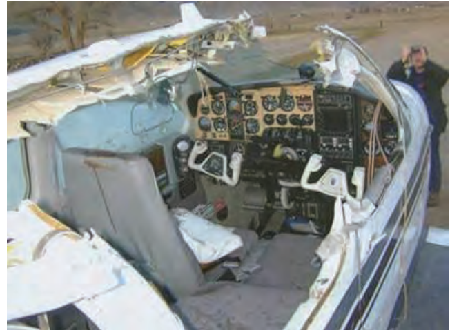
FIGURE 4 Canada Goose strike on GA aircraft (Source: Transport Canada).
