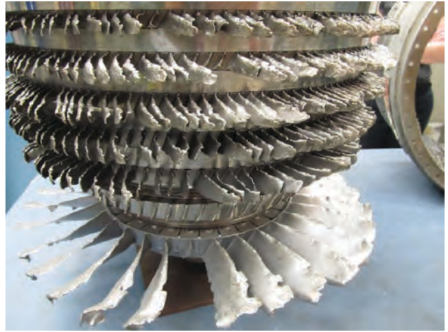
FIGURE 27 Jet engine destroyed by federal- and state-protected Burrowing Owl (Source: BASH Inc.).
