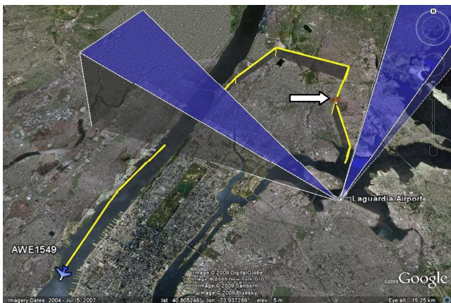
Figure 11: Portion of coverage pattern for V-array aligned to Runway 4 and to Runway 31. 1549 flight path is shown along with location of bird strike marked by arrow.
