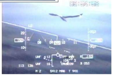
**Pilot's view.** Two pictures from an F-16 HUD (Head Up Display) video, showing a Herring gull flying in the path of the aircraft. The pilot did not have time for an evasive manoeuvre. With quicken wing-beat the Herring gull flew himself in safety.
