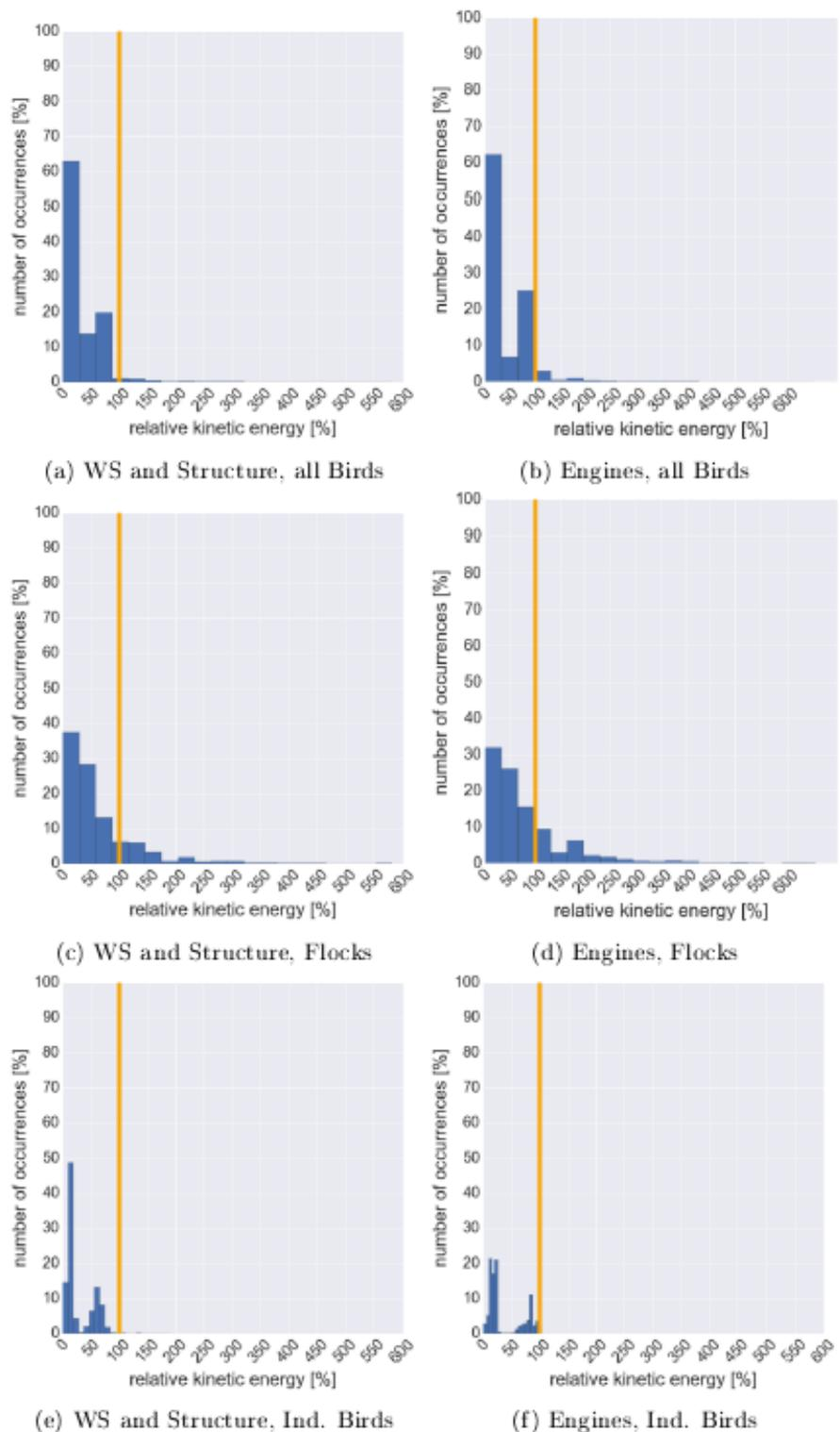
Figure 2. Distribution of kinetic energy for all birds, flocks and individual birds for the categories windshields (WS) and structure as well as engines (the orange bar represents the kinetic energy of the certification requirements).
